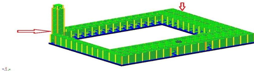
**Figure 7.** design model of the Great Mosque of Aleppo (condition before destruction).
