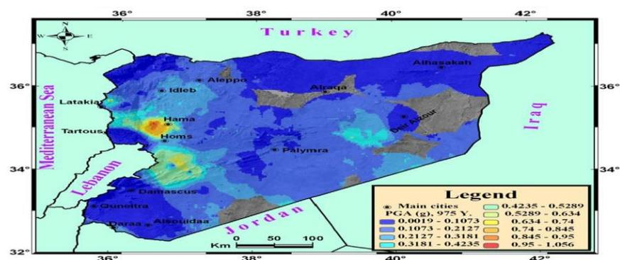
**Figure 4.** Map of the seismic hazard of Syria with PGA values in fractions of (g) for the earthquake return period of 975 (≈ 1000) years.
