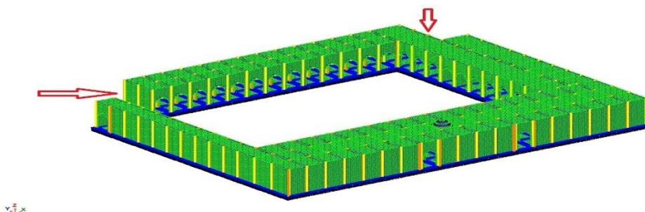
**Figure 8.** design model of the Great Mosque of Aleppo (condition after destruction). The arrows show the places of the main destruction.
