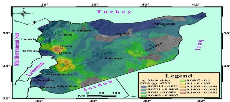
**Figure 3.** Seismic hazard map of Syria with PGA values in fractions of (g) for the earthquake return period of 475 (≈ 500) years.
