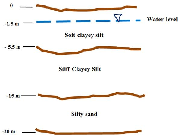
**Figure 4.** Soil Profile below the Minaret Foundation
