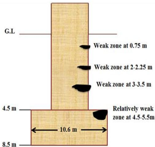
**Figure 21.** Weak Zones Location with the Minaret Foundation as Deduced from Seismic Crosshole Test
