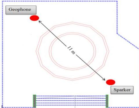
Figure 9. Borehole Geophone at Borehole -1 and Sparker at Borehole -2
