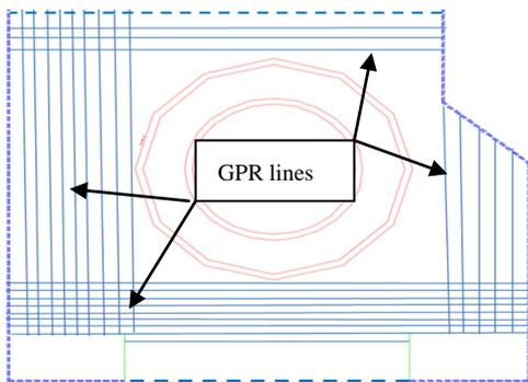
**Figure 5.** Locations of GPR Profiles around the minaret
