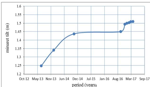
**Figure 2.** Measured Horizontal Movements of Minaret between 2013 and 2017
