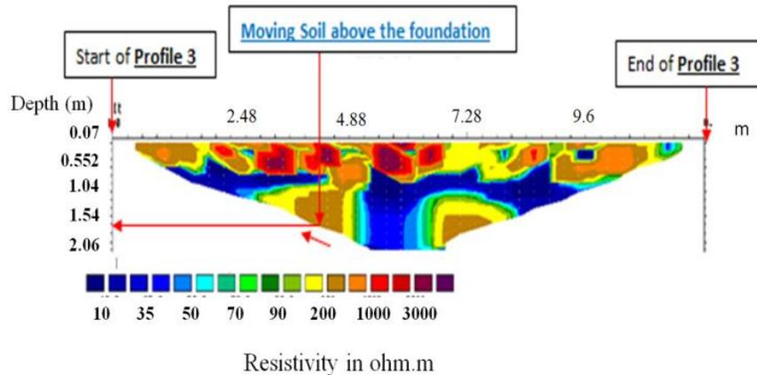
**Figure 16.** Apparent Resistivity in Profile 3
