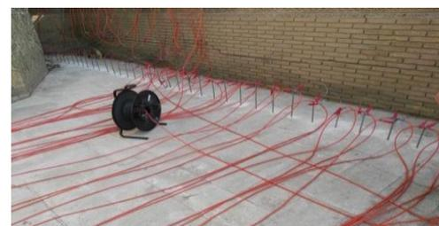
**Figure 8.** Electrodes Distribution at the Minaret Site
