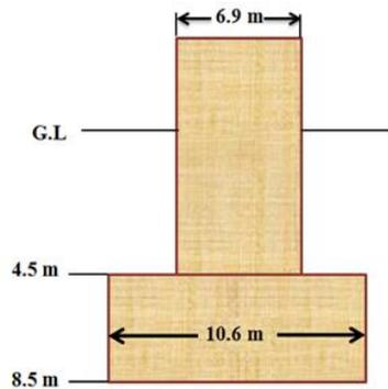
**Figure 20.** Shape and Depth of the Minaret Foundation belowground Level
