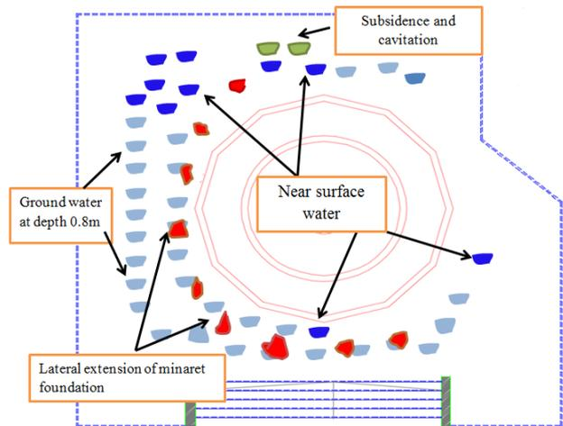
Figure 13. Main Subsurface Features of Soil Resistivity
