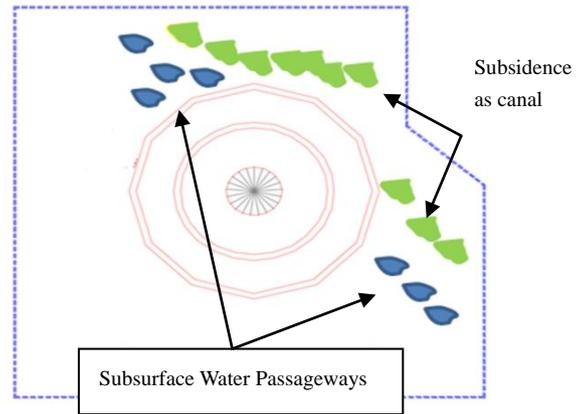
Figure 11. Main Subsurface Features that Detected by the GPR Survey: The Blue Spots Represented Subsurface Water Passageways and Green Represented loose Soil and Subsidence
