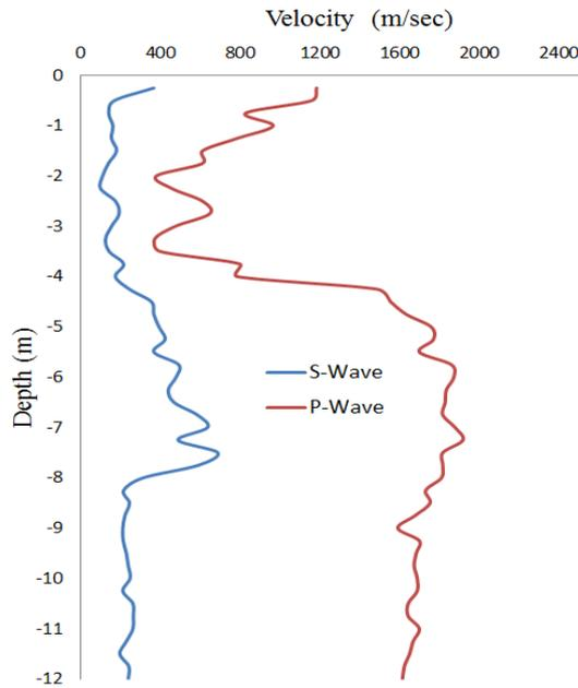
**Figure 18.** Variations of P-wave and S-wave Velocities with Depth
