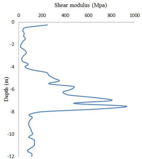
**Figure 19.** Variation in Dynamic Shear Modulus with Depth
