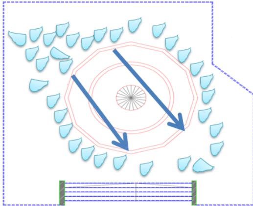
**Figure 14.** Possible Groundwater Movement Directions from Electrical Resistivity Test
