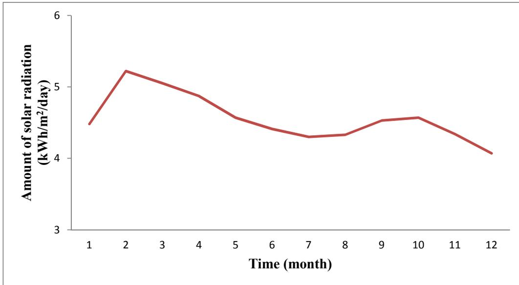
**Figure 1.** Monthly radiation incident average on a horizontal surface for 2008 (kWh/m<sup>2</sup>/day) [6]
