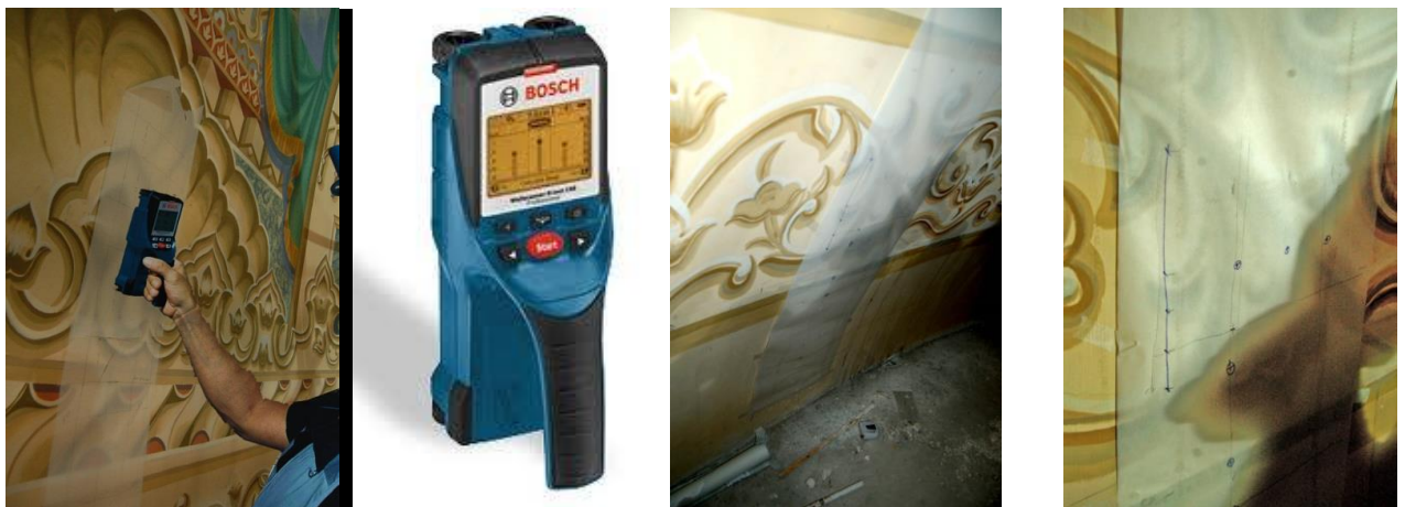
Figure 6. Rebar scanning equipment and application
