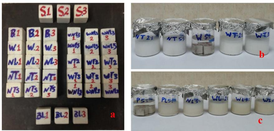
**Figure 7.** (a) The prepared cubic marble specimens and symbolized, (b) (c) specimens in consolidants.
