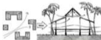
**WARM & HUMID CLIMATE:** Courtyards ratio is kept as 1:1 or in some case 1.5:1 in order to increase area for faster evaporative cooling.
