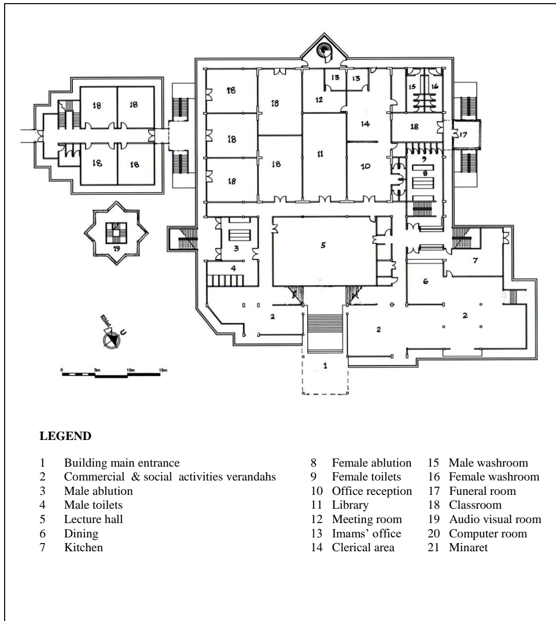
Figure 6.3: Ground Floor Plan of Masjid Saidina Abu Bakar As-Siddiq, Bangsar, Kuala Lumpur (1982). Source: Author
