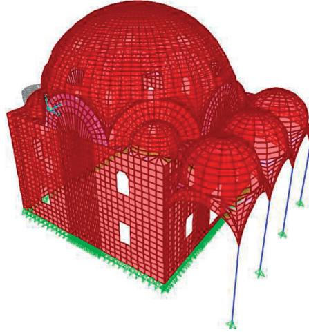
FIGURE 9: 3D FEM model of the Bajrakli Mosque.
