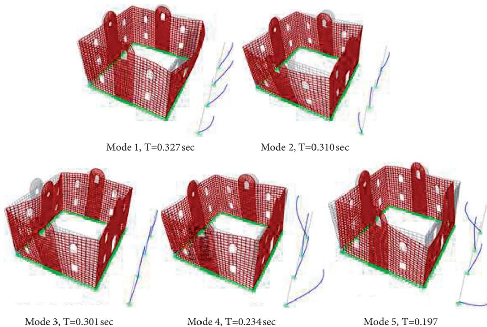
FIGURE 11: Modal shapes of the structure.
