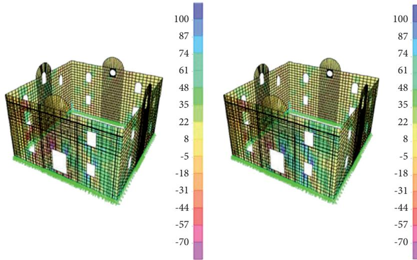
FIGURE 19: Shear stress distribution at load-bearing walls for (a)  $G + EQ_x$  and (b)  $G + EQ_y$ .
