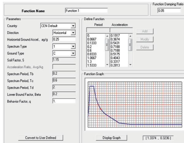
FIGURE 10: Response spectrum inputs.
