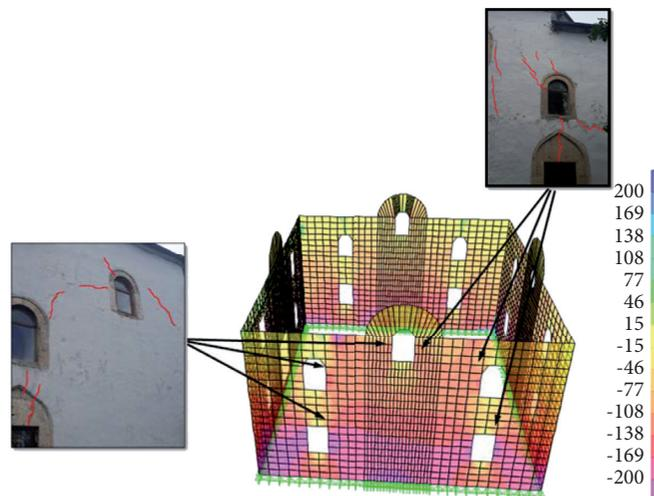
FIGURE 21: Comparison of visual inspections with finite element analysis for load-bearing walls ( $S_{22}-G + EQ_x$ ).
