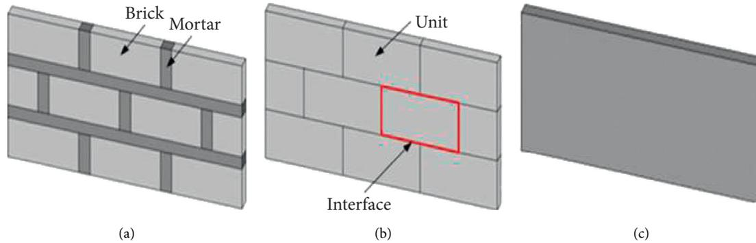
FIGURE 6: Masonry modeling approaches. (a) Micromodeling. (b) Mesomodeling. (c) Macromodeling [47, 49].
