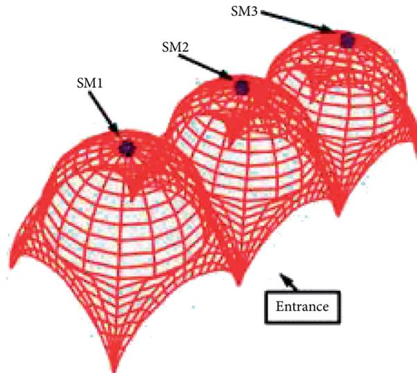
FIGURE 14: Location of the maximum displacements on the small domes.
