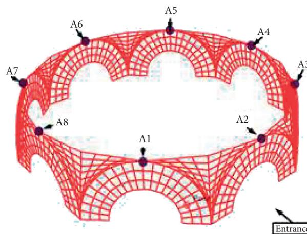
FIGURE 15: Location of the maximum displacements on the top of the main arches.
