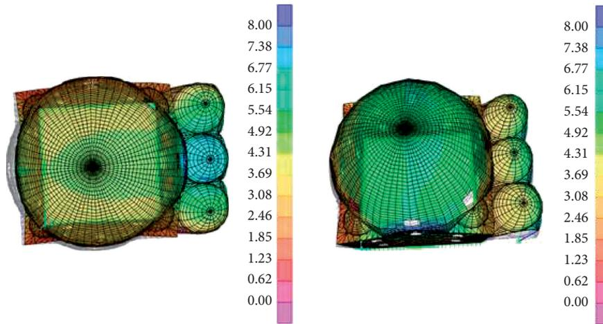
FIGURE 12: Maximum displacement for (a)  $G + EQ_x$  and (b)  $G + EQ_y$ .
