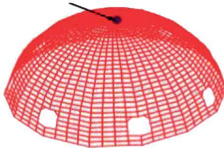
FIGURE 13: Location of the maximum displacements on the main dome.
