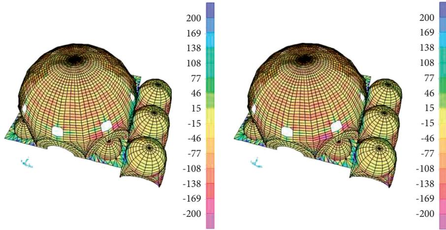
FIGURE 16: Tensile and compressive stress distributions at the roof system for (a)  $G + EQ_x$  and (b)  $G + EQ_y$ .
