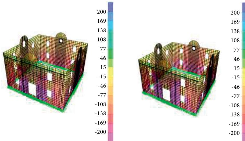
FIGURE 18: Tensile and compressive stress distribution at load-bearing walls for (a)  $G + EQ_x$  and (b)  $G + EQ_y$ .
