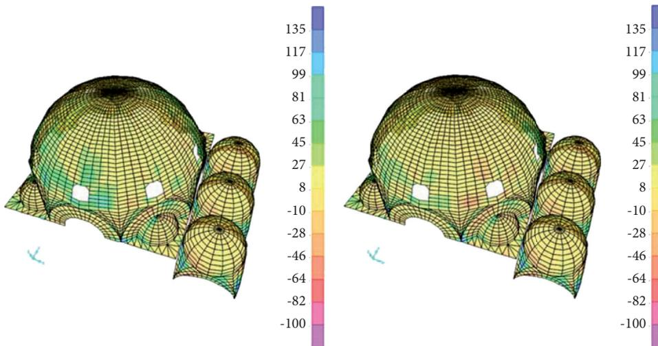
FIGURE 17: Shear stress distribution at the roof system for (a)  $G + EQ_x$  and (b)  $G + EQ_y$ .
