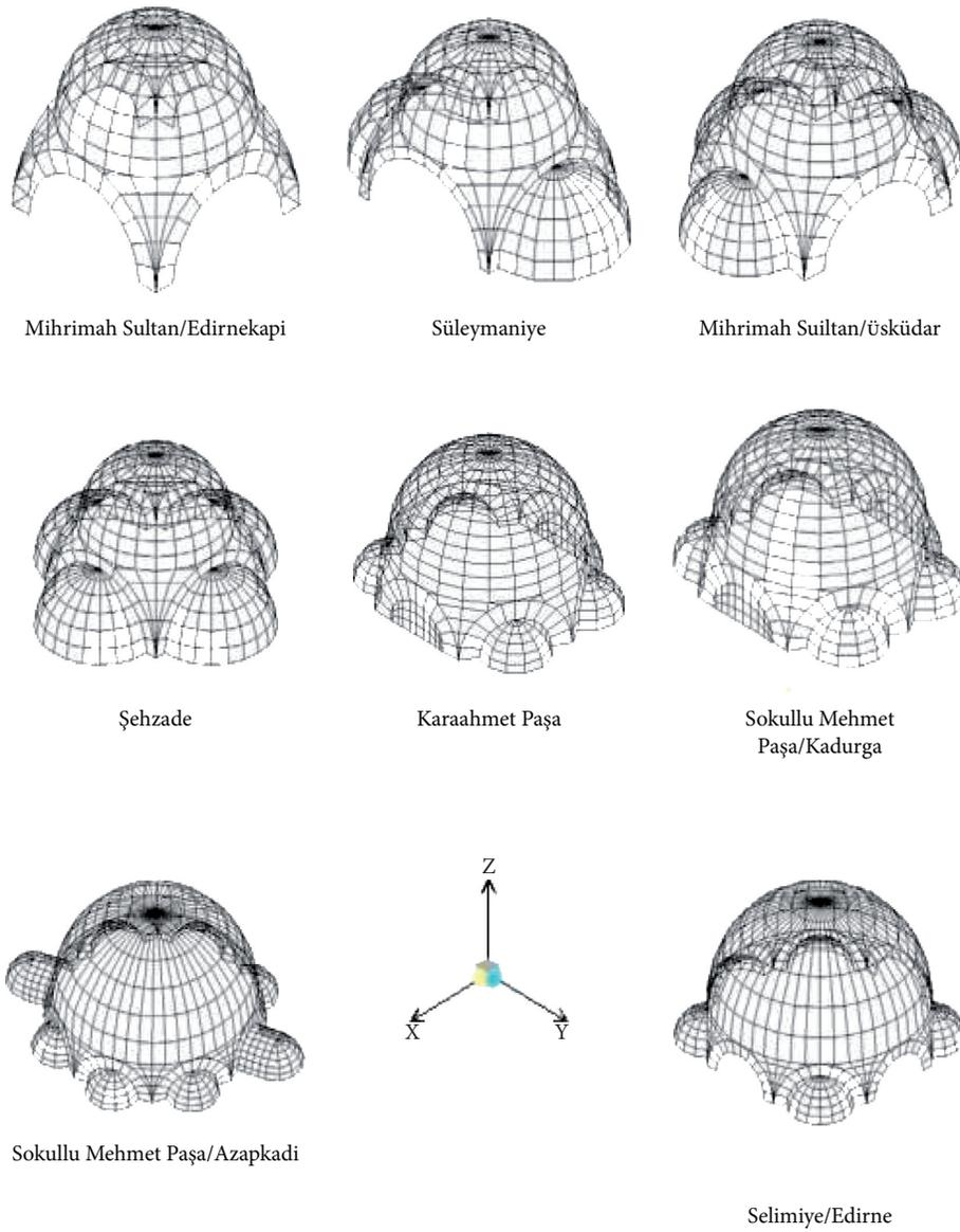
FIGURE 7: Finite element models of domed roof systems [25].
