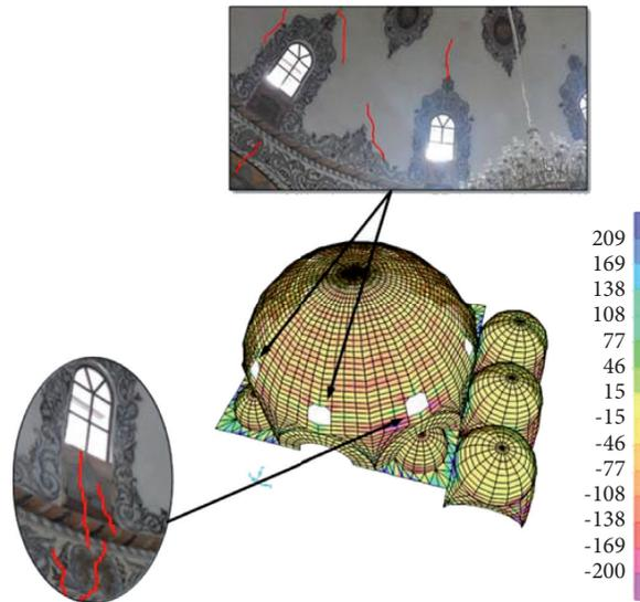
FIGURE 20: Comparison of visual inspections with finite element analysis for the roof system ( $S_{22}-G + EQ_y$ ).
