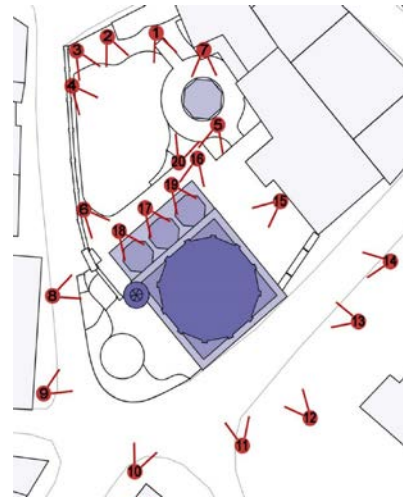
Figure 3. The schema of ground-based photogrammetric survey acquisition
