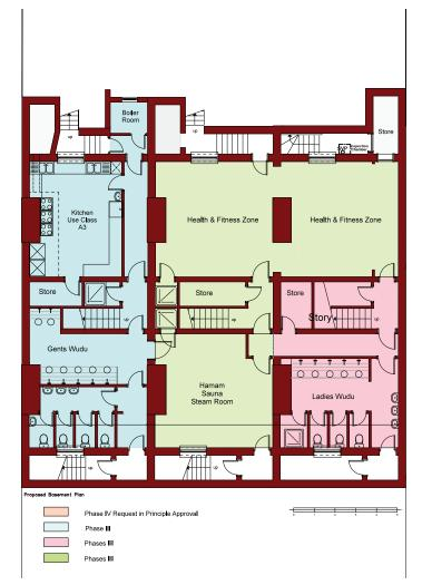
Fig. 104 - Proposed basement plan
