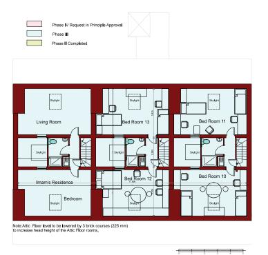
Fig. 108 - Proposed Attic Floor Plan
