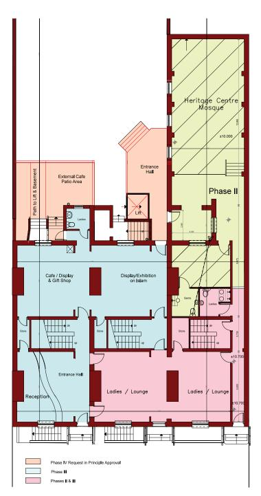
Fig. 105 - Proposed Ground Floor Plan
