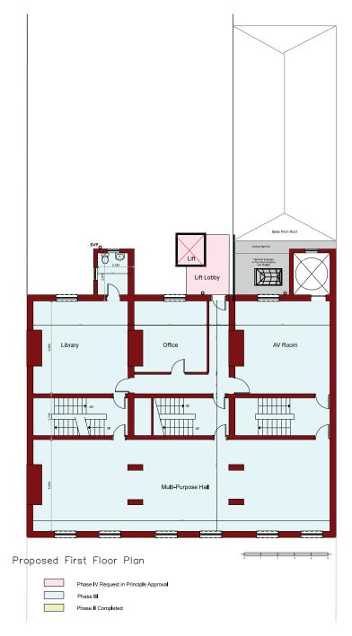
Fig. 106 - Proposed First Floor Plan
